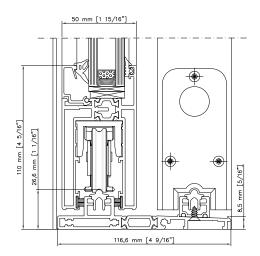
2 RAILS FLUSH THRESHOLD VERTICAL SECTION
