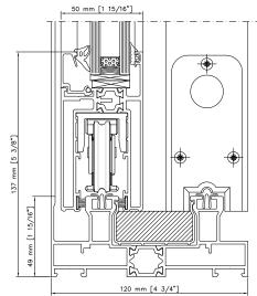
2 RAILS LOWERED THRESHOLD VERTICAL SECTION
